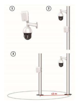
Figure 9-18 Scenario of One-Point Calibration
